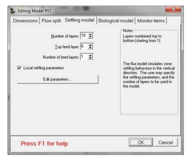
The settling velocity function parameters used for the model primary settling tank in this example are very close to those listed in the table above, with the exception of  $V_0$  and  $V_0$ , which were increased slightly to 300 m/d. The parameters used are shown below in US units:
