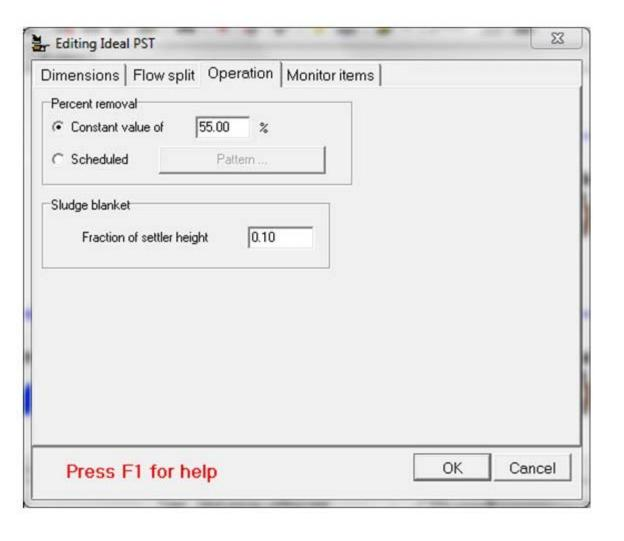
The model primary settling tank was set up with ten layers and Local settling parameters as shown below. If a model settling tank is used for both primary and secondary settling tanks in the same BioWin layout, then use of Local settling parameters is the safest way to ensure that the correct parameters are used in the various locations.
