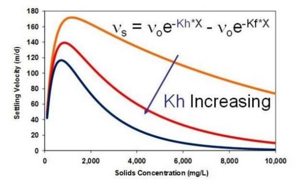
One advantage of the Double-Exponential model formulation is that it is quite flexible, and can be used to simulate a variety of different settling regimes that may be found in different types of settlers.
