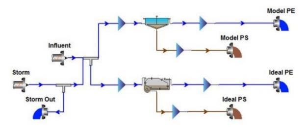
The layout includes two possible inputs: (1) a "typical" diurnal influent pattern named Influent, and (2) a "storm" input named Storm that if allowed to enter the process results in the total flow directed to each primary settling tank being doubled and the load increasing by 50%. Whatever flow is allowed into the process is divided equally between the two primary settling tanks. A number of general mixers are used in the layout to help with plotting inputs and outputs.
