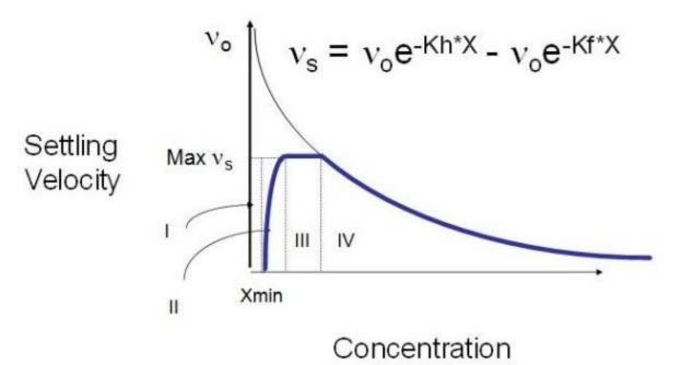
where  $V_0$  = maximum Vesilind settling velocity, Kh = hindered zone settling parameter, Kf = flocculent zone settling parameter, and X = is the total suspended solids concentration.
