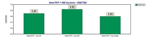
The VSS/TSS ratio of the primary effluent has *increased* to 0.92 and the primary sludge ratio has *decreased* to 0.80 due to the additional ISS capture.
