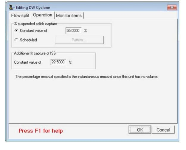
A dewatering cyclone applies the specified % solids capture rate to the incoming mass rate for *all* particulate state variables (including ISS) in the same way of a "normal" solid/liquid separation element. The captured solids are directed to the underflow stream, and the remainder report to the overflow stream.
