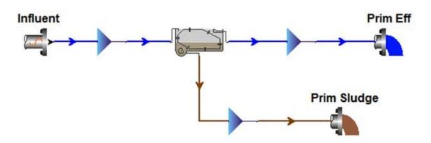
Four our base case, we'll use the simple ideal PST element shown above. The charts that are plotted in the Album of the BioWin file for our base case (<u>Base Ideal PST #1-Base Case.bwc</u>) have been generalized such that they rely on the mixing elements on the PST influent, underflow, and effluent streams. This means that it is very easy to modify the file that comes with this article and not disrupt the charts.
