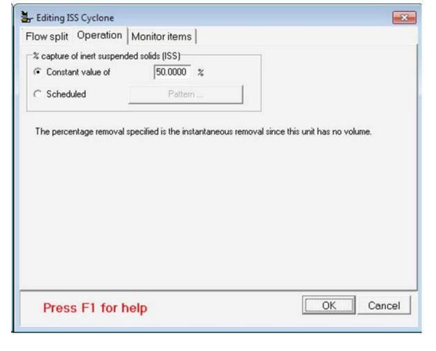
In a "normal" BioWin solid/liquid separation element, we specify a % solids capture, and this capture rate is applied to the incoming mass rate for *all* particulate state variables. The captured solids are directed to the underflow stream, and the remainder report to the overflow stream.
