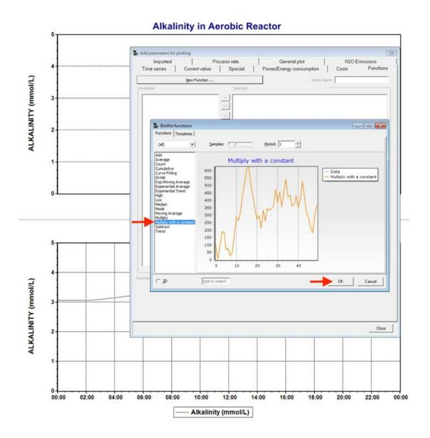
Select the **Alkalinity (mmol/L)** series from the **Available** list and use the right-pointing arrow to bring it to the **Selected** list. Name this function series **Alkalinity (mgCaCO3/L)**. At the bottom of this window, type **50** beside the "Multiply by". Click close to add this function series to the graph.
