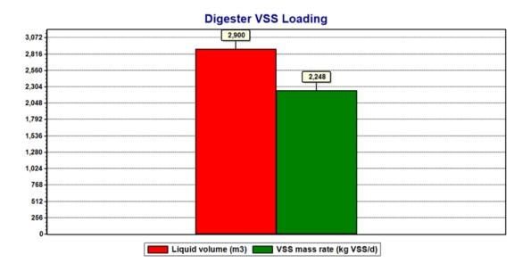
Add a function series to divide the VSS mass rate by the digester volume. Right-click on the Current Value plot and select **Add Series** in the resulting popup menu. On the **Functions** tab, we click the **New Function...** button, select the **Divide** function and click the **OK** button.
