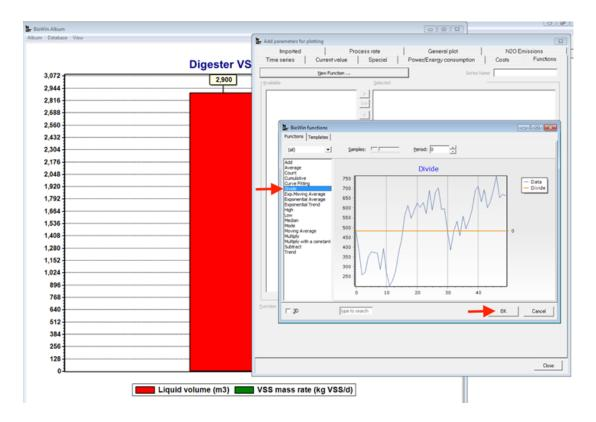
We first bring the VSS mass rate (kg VSS/d) series from the Available list to the Selected list. Next, bring the Liquid volume (m3) series to the Selected list. When applying the Divide function, the series at the top of the Selected list (VSS mass rate (kg VSS/d)) will be divided by the series below (Liquid volume (m3)). Name this function series Loading (kg/(m3 d)). Click close to add this function series to the graph.
