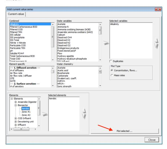
On the bottom, add a time series chart, select **Alkalinity** from the Combined variables list and select **Bioreactor > Aerobic** from the Elements list. Click "Plot selected" to close the window.
