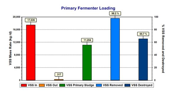
The dewatering unit used to separate the solids from the liquid in the fermenter has a specified solids removal of 99.4%. The function series **VSS Removed** that we have plotted in the BioWin album shows that the VSS removed across the fermenter-thickened-sludge loop is actually 98.2%.
