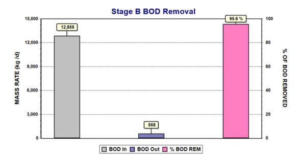
The BOD removal across the A-stage in our BioWin model is 63.3%, which is slightly higher than the typical range of 50% to 60% (Bohnke, 1990). Almost all of the remaining BOD is removed across the B-stage (95.6%), which is expected because the B-stage has a relatively long SRT.
