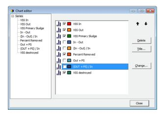
We can format our chart as desired. When we place our cursor over the Primary Sludge Fermenter on the BioWin flow sheet, we see in the bottom right summary pane that the steady-state VSS destruction is 10.2%. However, the function series **VSS Destroyed** that we have plotted in the BioWin album shows that the VSS destruction across the fermenter-thickened-sludge loop is actually 65.7%.
