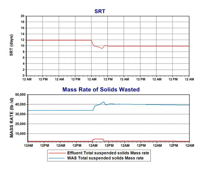
Finally, let's look at the effluent response to taking one train offline. The shift of solids out of T2 and into the clarifier results in a spike in the effluent solids concentration (see effluent TSS profile below) since settling performance is impacted by the higher solids loading rate. Twenty-four hour flow weighted composite effluent TSS concentrations show a small increase to approximately 13.7 mg/L TSS during the period when T2 is taken
