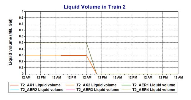
Since we also incorporated a schedule into the feed splitter the changes in operation can be easily tracked by plotting the flows in this splitter. We see at 12AM on the third day of operation the flow to the second train T2 (represented by the underflow of the feed splitter or the series called Flow to Train 2) falls to zero and the flow to the first train (represented by the main flow of the feed splitter or the series called Flow to Train 1) increases by
